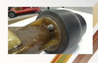
Materials used: Hemp-agave mat, fibreglass mat, polyurethane foam
