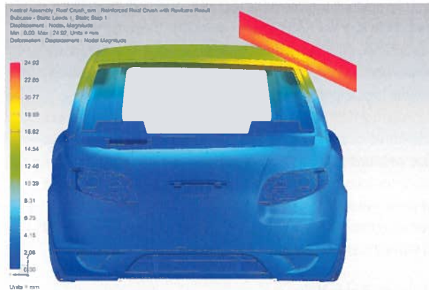
Roof crush analysis of the Kestrel concept vehicle.
